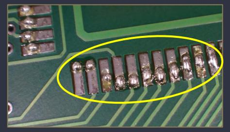
**How to Recognize:** Both nonwetting and dewetting can be visually identified. Nonwetting will show areas where the solder has not bonded to the surface at all. Dewetting will show areas where solder initially bonded but then pulled back, leading to exposed base material and a rough, irregular solder finish.
