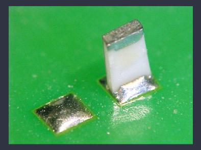
**How to Recognize:** Tombstoning can be visually identified by observing components such as resistors or capacitors standing vertically instead of lying flat against the PCB. The defect is more prominent with 0402, 0201, or smaller component sizes.
