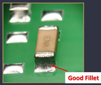
**How to Recognize:** Insufficient solder can be visually identified by observing that the solder joint appears incomplete or not fully formed. The solder might not have completely covered the pad, or the fillet might appear shallow or non-existent. The joint may also lack the typical concave shape at the component lead-to-pad interface.
