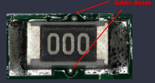
**How to Recognize:** Solder beading can be visually identified by spotting tiny solder balls positioned near the ends of chip components. These beads are typically larger and more defined than the more randomly dispersed solder balls caused by balling or spattering.
