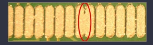
**How to Recognize:** Bridging can be visually identified by observing solder connections between two adjacent pads or leads where there shouldn't be any. These connections can appear as thin solder filaments or broader solder masses spanning between pads.
