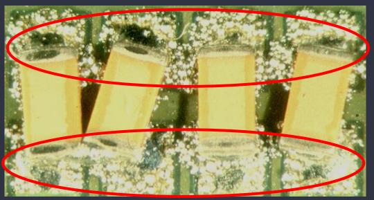
**How to Recognize:** The defect can be visually identified by observing a solder joint that appears rough, granular, or matte instead of the typical smooth and shiny appearance. Under magnification or X-ray, unreflowed solder particles might be visible within the joint.
