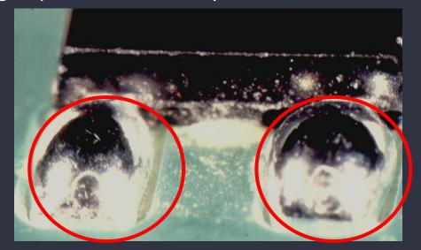
**How to Recognize:** The defect can be visually identified by observing a solder joint that appears larger and bulkier than typical. The fillet might extend significantly up the component lead or even touch the component body. In severe cases, the excessive solder might form bridges or shorts with neighboring components or traces.
