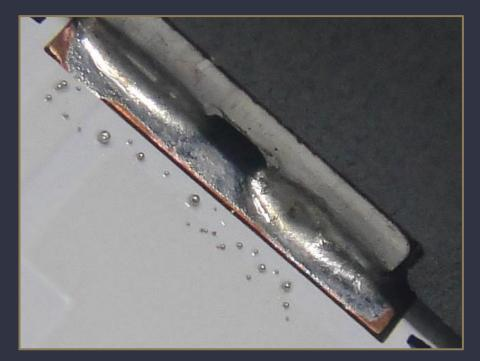
**How to Recognize:** Solder balling can be visually identified by the presence of small, round solder beads on or around the soldered areas of the PCB.
