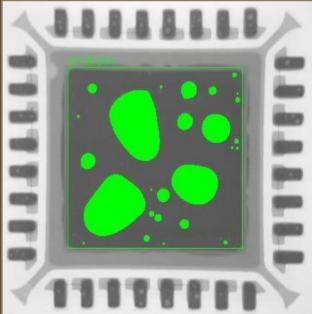
**How to Recognize:** Voids are typically not visible on the surface of the solder joint. They are most commonly detected using X-ray inspection, where they appear as dark spots or areas within the X-ray image of a solder joint.
