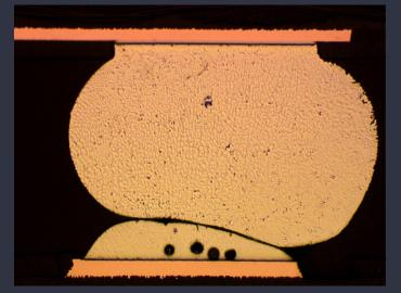
**How to Recognize:** In general, NWO can be identified visually by observing a clear gap or separation between the solder and one (or both) of the connection pads. It's best recognized using X-ray inspection, where the solder ball and solder paste appear distinct, lacking the expected coalescence. The defect often manifests as an intermittent electrical connection.
