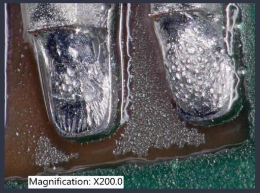
**How to Recognize:** Grainy joints can be visually identified by the distinct granular texture on the solder joint surface.
